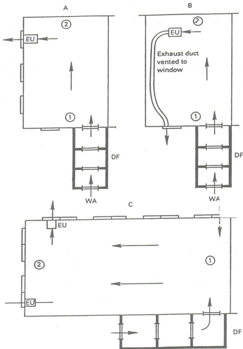
DF- Decontamination Facility; EU – Exhaust Unit; WA – Worker Access; A – Single room work area with multiple windows; B – Single room work area with one window; C – Large single room work area with windows. Arrows denote direction of air flow. Circled numbers indicate progression of removal sequence.
