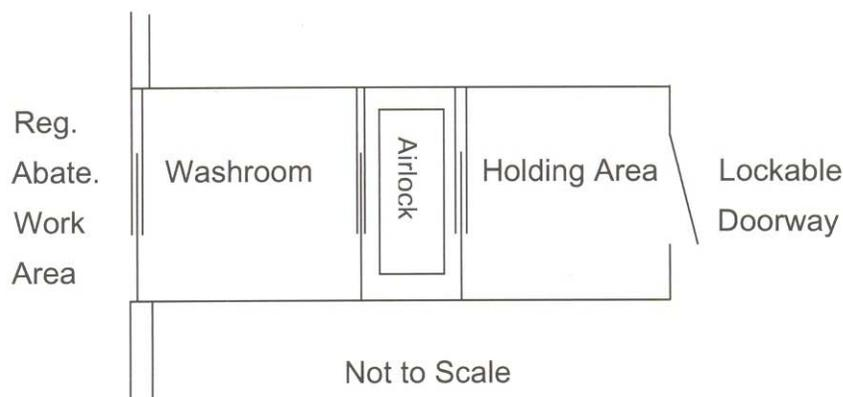
All waste and equipment exiting the work area must pass through the waste decontamination system prior to being removed from the site. External surfaces of asbestos waste bags and wrapped debris, as well as all tools and other equipment must be wet wiped and/or HEPA vacuumed in the work area before being permitted to exit the site.
