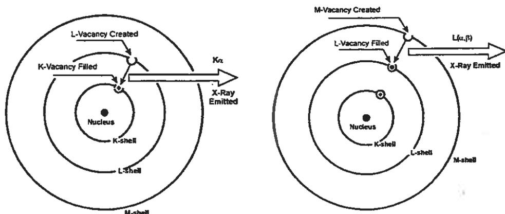
**Figure 5-3. Illustration of electron shell vacancies and filling**
