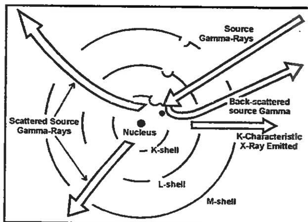
Figure 5-6. Scattering of the source gamma rays
