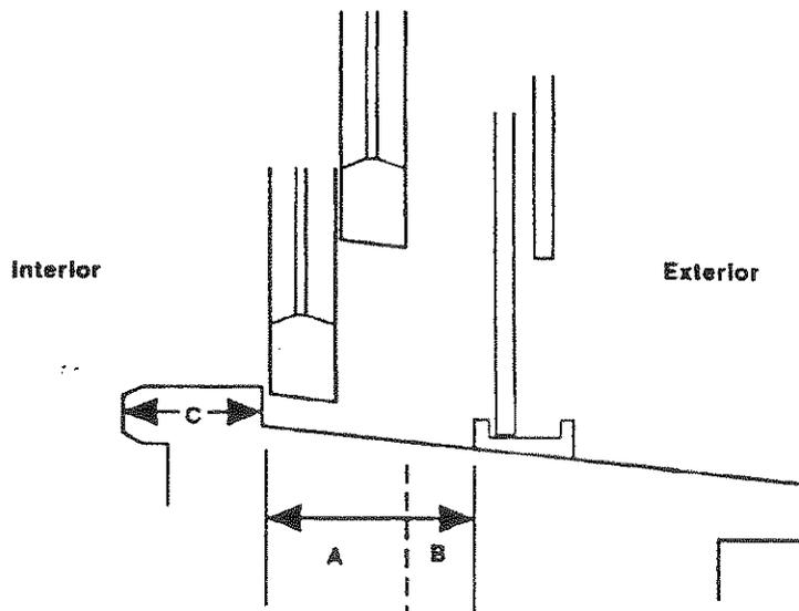
2. Side view of window (including storm window) showing window trough area, A and B, to be tested. Trough extends out to storm window frame. The interior window sill is shown as area C. Interior window sills and window troughs should be sampled separately.
