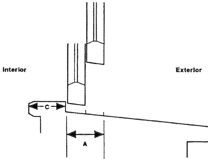
1. Side view of window (with no storm window) showing window trough area, A, to be tested. Trough is strip across window sill where interior window sashes can touch the sill. The interior window sill is shown as area C. Interior window sills and window troughs should be sampled separately.
