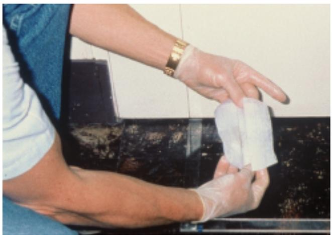
FIGURE 5.11d Folding wipe over for second pass.
