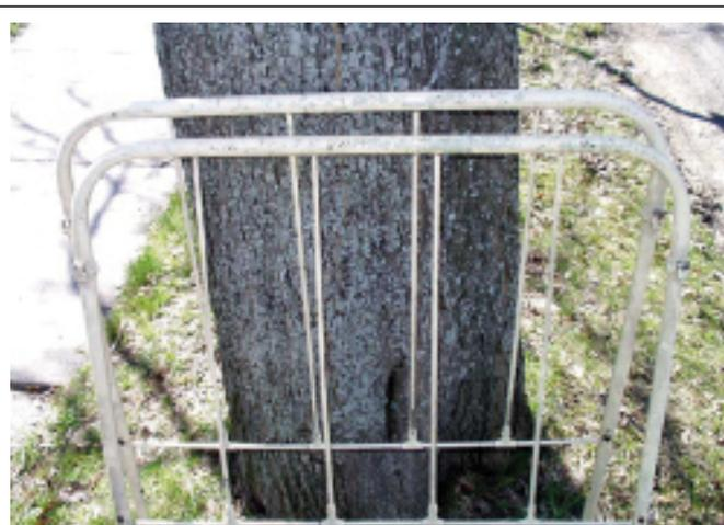
**FIGURE 5.18** Baby's bed exhibiting deteriorated paint and evidence of teeth marks.
