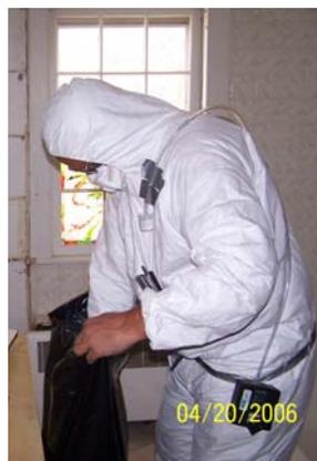
**Figure 3.2 - Photograph of a PBZ Air Sample on an R&R Worker**
